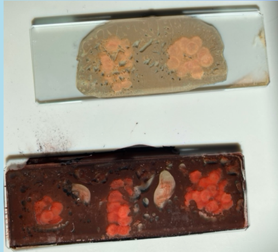
Two SPMU inks responded to the laser energy by becoming lighter in colour.
